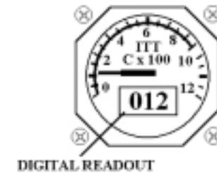
The ITT system is the indication system for the turbine gas temperature. The system measures the engine gas temperature at the station between the low pressure turbine and the high-pressure turbine inlet. Analog and digital readout is given in degrees centigrade.
