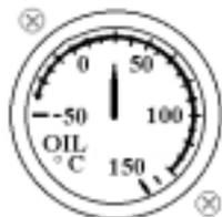
The Oil Temperature Indicator shows the oil temperature in the engine. Temperature is given in degrees Celsius.
