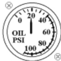
The Oil Pressure Indicator shows the oil pressure in the engine. Pressure is given in PSI (Pressure per square inch).
