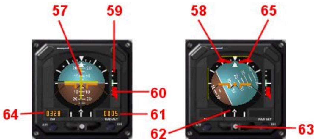
Attitude provided with electrical power and pressure
