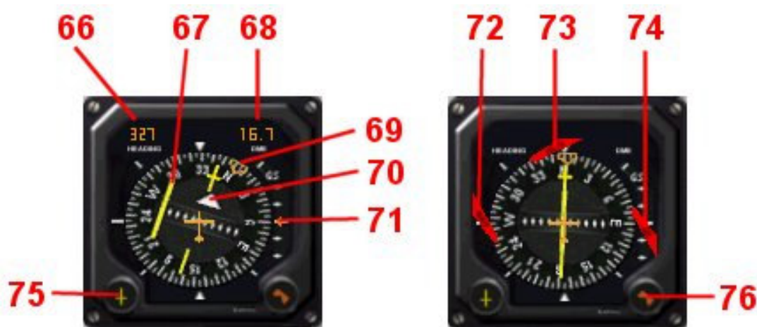
HSI provided with electrical power.
